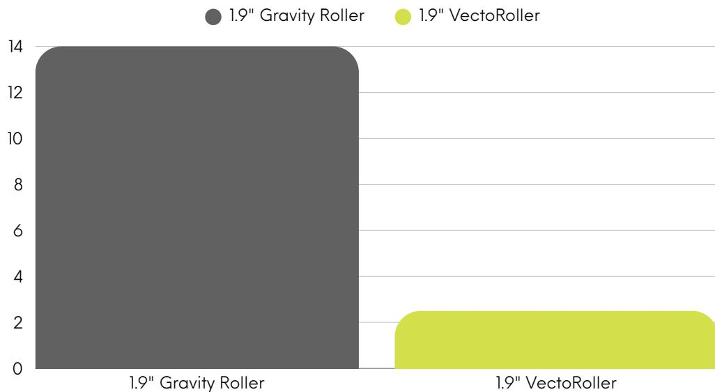
In controlled testing, a 50 lb plastic tote required approximately 14 lbs of lateral force to move across a standard 1.9" gravity roller, compared to approximately 2.5 lbs when using the Vectoroller™. Results reflect test conditions and demonstrate the potential impact of reducing lateral friction at the roller surface.
